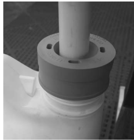
Figure 7. Laundry adapter fitting on standpipe, fit onto chemical drum opening.
